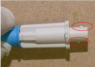
5.2 Prime the Digitail Injector by depressing the end cap. A metal rod will protrude 2cm.
